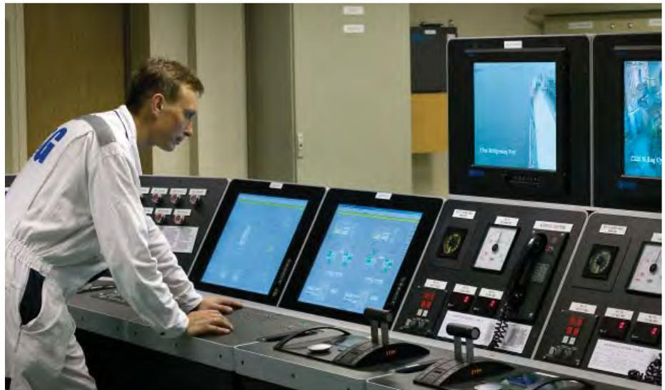
*Picture: Kongsberg's K-Chief 500, alarm, monitoring and control system, which can be integrated to the Neptune Engine Room Simulator.*
