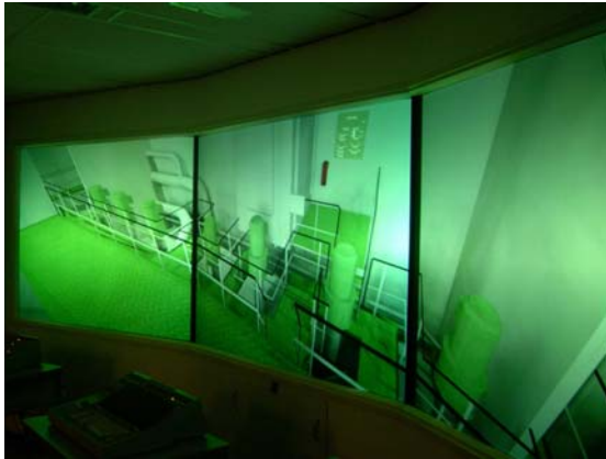
Virtual Engine Room integrated with the real engine room simulator, see section 1
