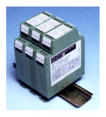
junction). A built-in temperature sensor will compensate for variations in the amplifiers ambient temperature (cold junction). Two independent amplifiers are built in the same terminal block housing.
