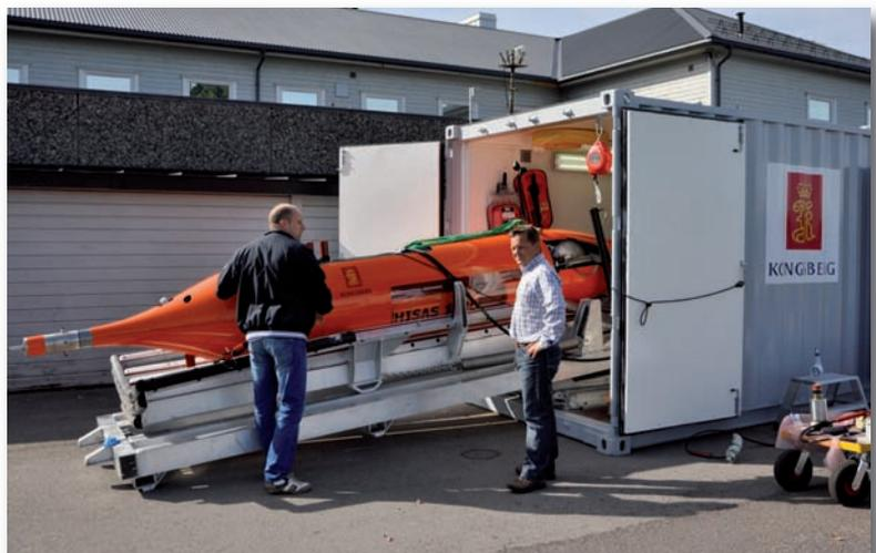
*HUGIN 1000 AUV Resting on L&R System (Stinger) Extended from the 20-Foot Container*
