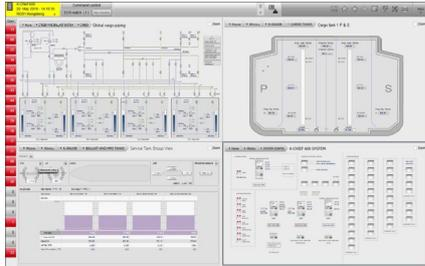
Figure 8: Tank monitoring system mimics (split screen example)
