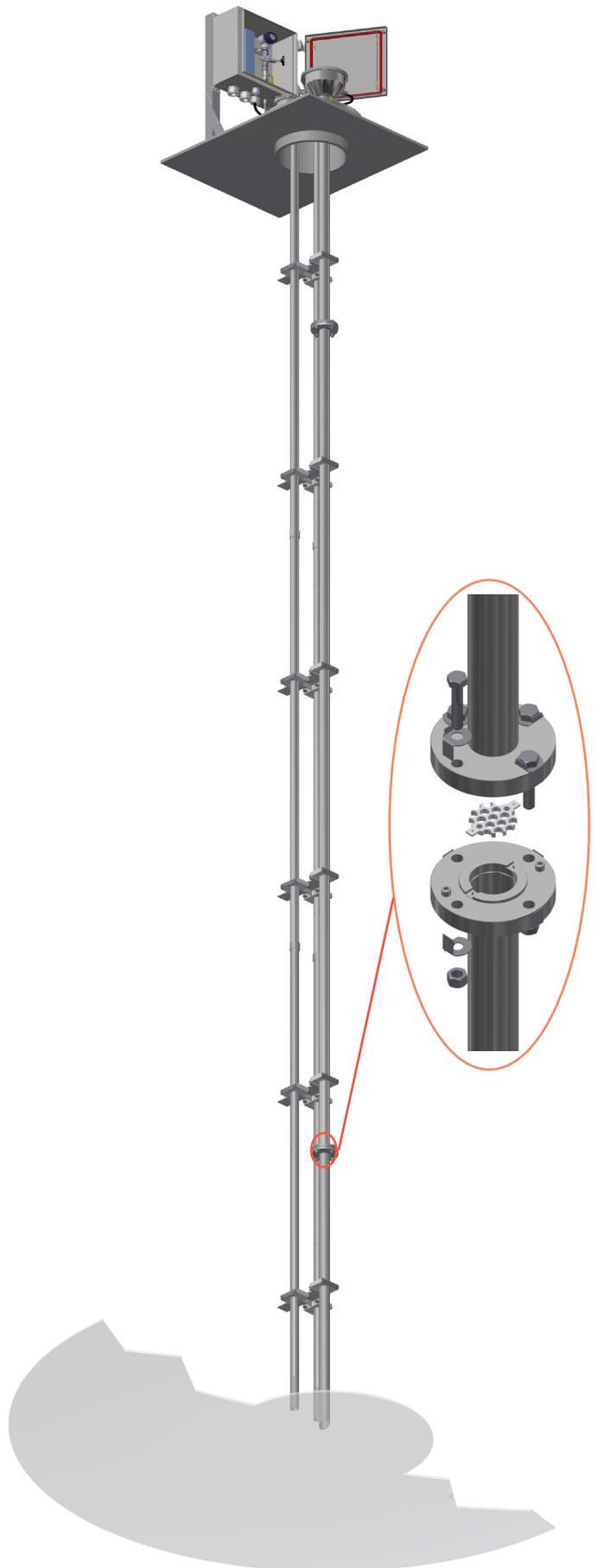
Figure 7: Standpipe installation with marker for auto-calibration by
