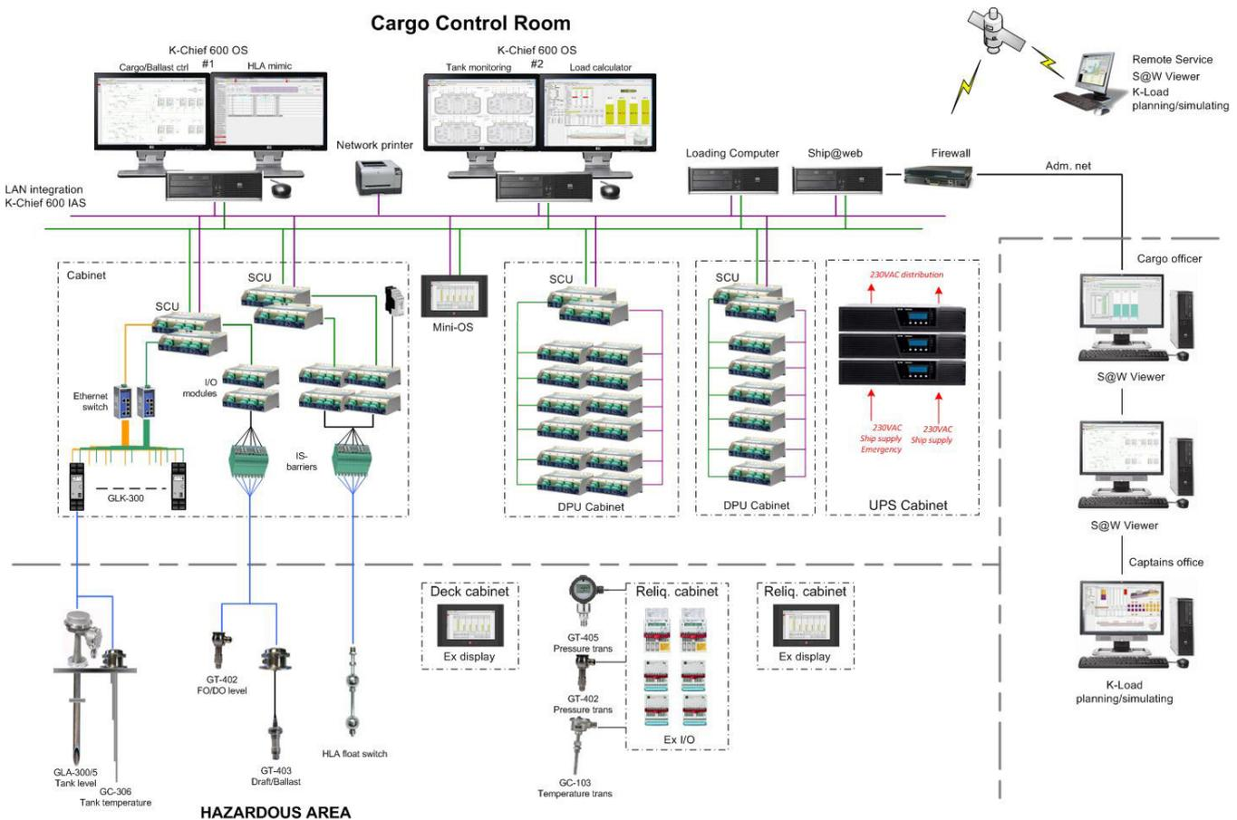
Figure 9: KM integrated LPG tank management topology
