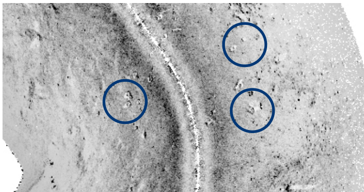
GeoSwath Plus Compact 500 kHz geo-referenced side scan data collected in 5 m water depth in a Kleipeda port, showing debris including car tires.
