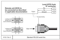
This cable comprises a multi-purpose serial line. It provides interface with any peripheral unit. One end of the cable connects to the local unit (DTE) with a 9-pin 'D' connector, while the other connects to the peripheral (DCE) as described in the peripheral unit's documentation
