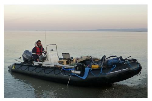
Survey vessel, an inflatable craft with the GeoSwath Plus Compact sonar head installed on a retractable pole together with peripheral sensors, motion reference unit, GPS and sound velocity probe. The splash protected deck unit is powered by batteries and operated via a ruggedized laptop.
