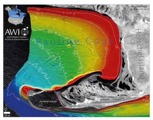
Bathymetry map of Pauline Cove on Herschel Island, YT, Canada. The area was chosen as the natural laboratory for coastal erosion processes in permafrost regions. The bathymetry is the baseline for long time studies. Note the dredge marks caused by sea ice processes.
