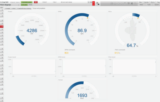
Integrated to K-Chief – AutoChief sequence view including torque and power information
