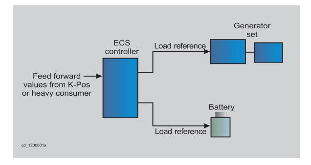
Load fluctuations handled by DLP combined with Energy Storage System (ESS) control:
