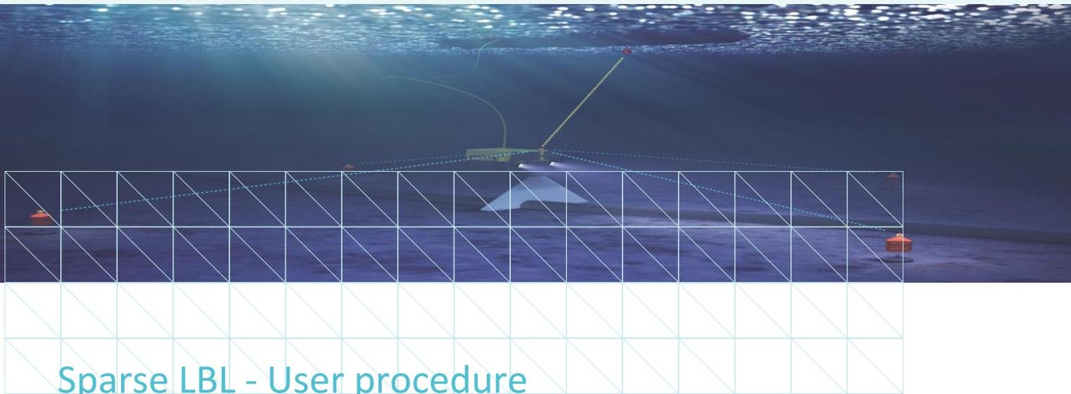
Sparse LBL enables LBL positioning of an ROV using only two cNODE seabed transponders. This function can be combined with HAIN.
