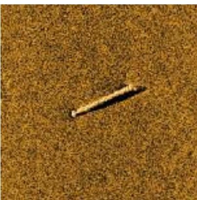
Standard FOCUS streaming SAS image (20 m x 20 m) of torpedo at 90 m range.
