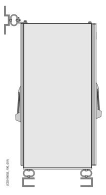
Use bulkhead support bracket(s) to make installation easier, and/or "U" shaped profiles to make more space for cables under the cabinet.
