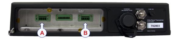
A P1: Transducer: Channel 1 - 2B P2: Transducer: Channel 3 - 4
