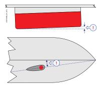
• Each transducer must be mounted with a small inclination angle (approximately 2 degrees).
