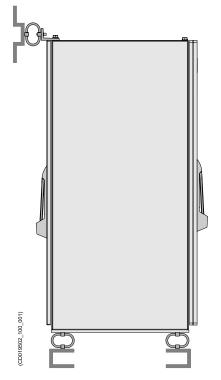
Use bulkhead support bracket(s) to make installation easier, and/or "U" shaped profiles to make more space for cables under the cabinet.
