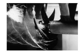
caused by the propellers. Propeller cavitation is a severe source of noise. The cavitation starts when the water flows in the same direction as the propeller blades. This is where the propeller blades move downwards.
