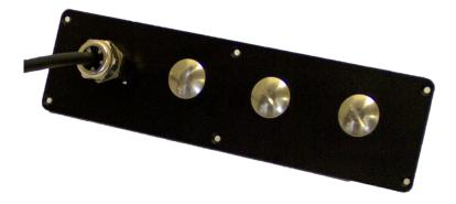
13 Connect the conductors in the transducer cable to the correct pins in the plugs, using the pin-out and the ship's cable plan. Check the license information to see which transducer to install where.
