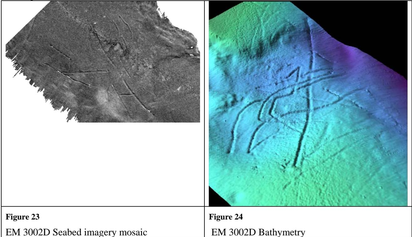
The multibeam seabed imagery data is geometrically correct and with good resolution, only slightly smoother than the EA 400 sidescan. Also the bathymetric data set gives a good description of the anchor drag marks.
