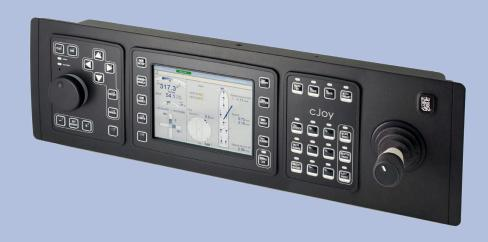
The cJoy Operator Terminal MK3 serves as the main operator interface for the cJoy Compact Joystick system. The terminal is a user-friendly tool for joystick, station keeping and autopilot operation.
