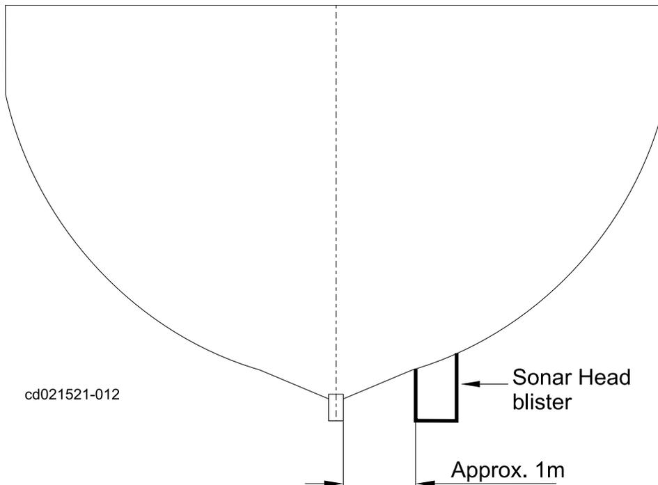
The interior of the blister should be filled with sea water by provision of a drainage hole in the bottom and an air outlet on the top. It is an important security precaution to have water pressure behind the head to counterbalance the outside pressure during vessel pitch in a rough sea.
