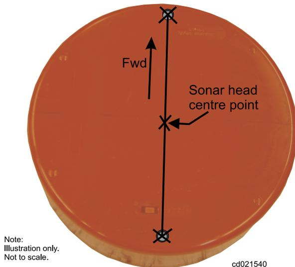
A ruler oriented with the face index marks can be used to give the heading and pitch of the Sonar Head. By making the ruler as a right-angle cross the roll may be measured.
