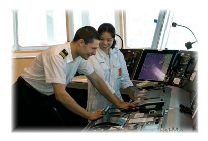
The Alarm and Command Panel (ALC) is a specially designed operator panel for the K-Chief 600 Marine Automation System in the bridge environment.
