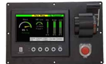
The TFT technology gives good visibility in night and daylight. The illuminated Lever has 11 telegraph positions with well defined notch in each position. Emergency Stop Switch is independent of panel and connected directly to Main Engine Safety System.
