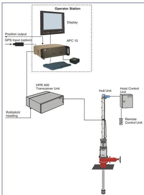
the transducer and hull unit. The system can be configured with one or two hull-mounted transducers. With the use of two transducers, flexibility and redundancy will be further improved. The system is controlled and operated from an Operator Station (OS) using the APOS software. The APOS software runs on a Windows XP platform, using standard windows graphical user interface.
