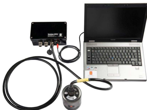
MRC+ connection setup with junction box
