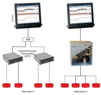
Colour LCD display with built-in CPU, One or two transceivers units for dry area environment (IP40), each with one or two transducers.
