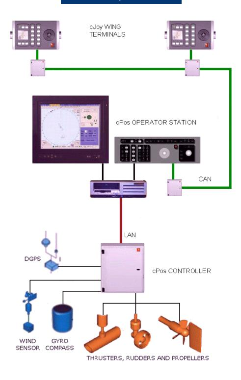
cPos used as a DP control system with main operator station and additional bridge wing terminals.
