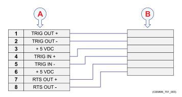
**A** Local connection The connector is RJ45 type.
