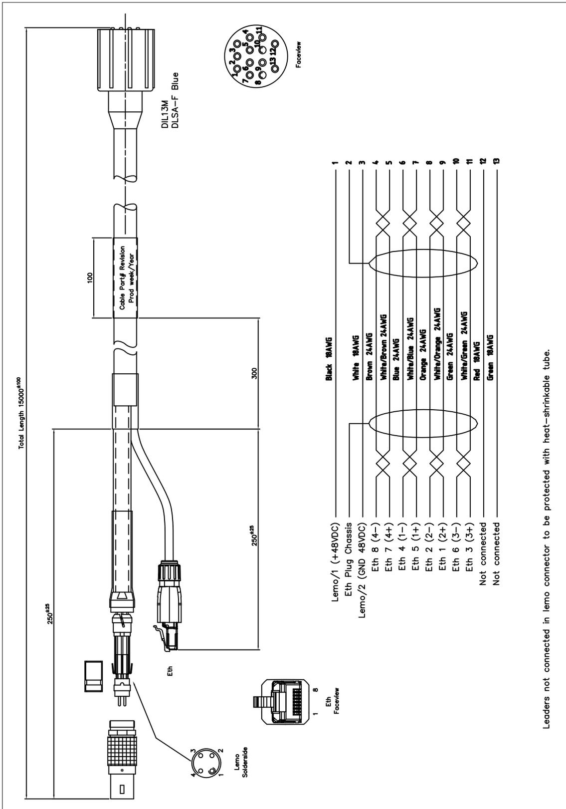
Leaders not connected in lemo connector to be protected with heat-shrinkable tube.
