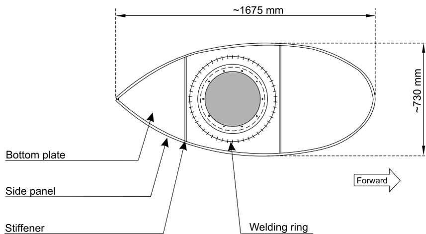
Figure 4 Blister arrangement - example for dual head
