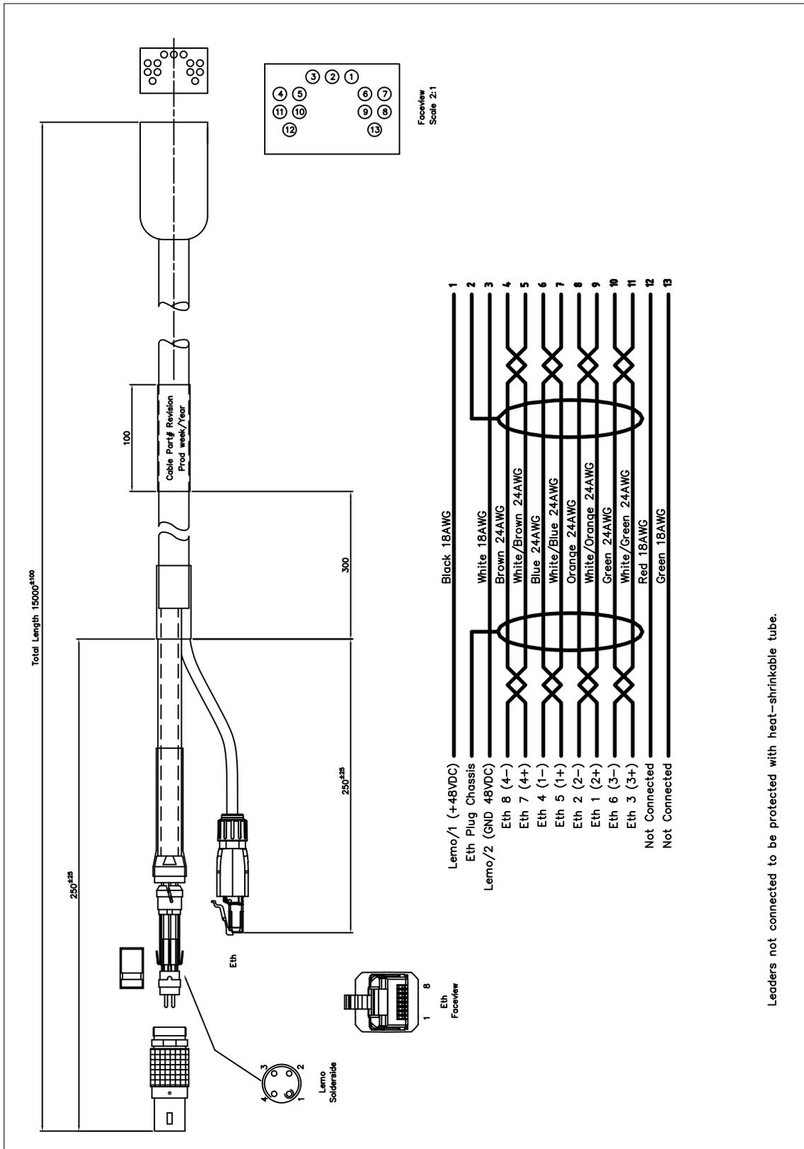
Leaders not connected to be protected with heat-shrinkable tube.
