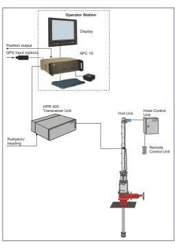
the transducer and hull unit. The system can be configured with one or two hull-mounted transducers. With the use of two transducers, flexibility and redundancy will be further improved. The system is controlled and operated from an Operator Station (OS) using the APOS software. The APOS software runs on a Windows XP platform, using standard windows graphical user interface.
