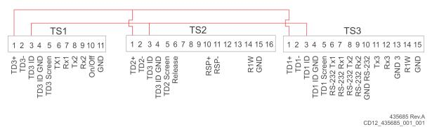
The transducer signal between TD1, TD2 and TD3 is linked on the terminal blocks.
