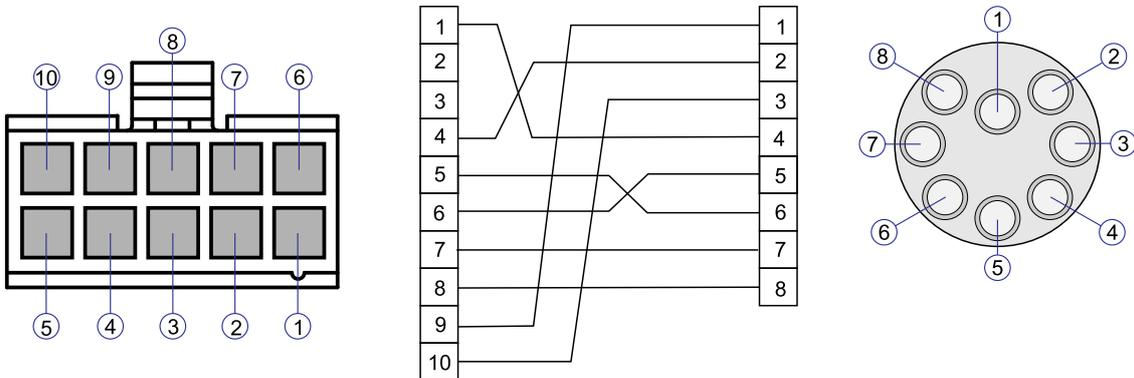
This is the Molex plug seen from the back where the crimp terminals are installed and a face view of the connector.
