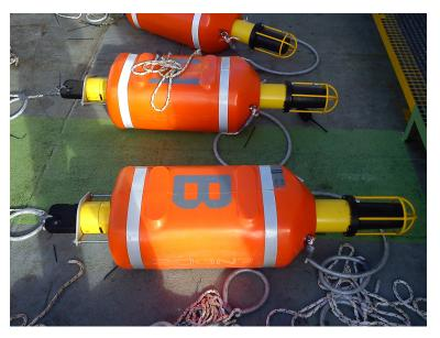
The transponders are rated to 6000 metres, depending on housing. The transponders are designed with a modular construction which means that the transducer, transponder electronics, battery pack and optional add-on's can be replaced individually to suit the operation.
