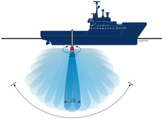
The HiPAP® 351 has a spherical transducer with a cylindrical body including 46 transducer elements. This model has good accuracy in the  $\pm 60^\circ$  sector and is suited for operations where the major positioning objects are within this sector. The total coverage is  $\pm 80^\circ$ .
