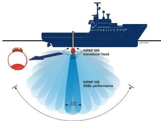
The HiPAP® 450 transducer is the same unit as the HiPAP® 500 transducer. The system has Transmitter/Receiver boards for only 46 elements, similar to the HiPAP® 351 system.
