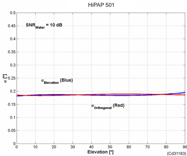
The figure above shows the accuracy as a function of elevation angle. The signal to noise ratio of 10 dB is in the bandwidth.
