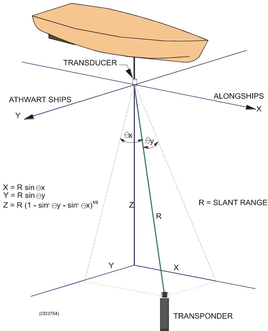
Figure 2 SSBL principle
