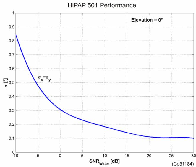
The figure above shows the accuracy as a function of signal to noise ratio. The elevation and the orthogonal angles are  $0^\circ$  (at vertical).
