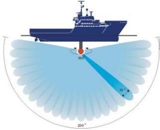
The HiPAP® 501 has a full spherical transducer body including 241 transducer elements. This model has close to full accuracy in the half sphere sector and is the preferred system where the best possible performance is required. The HiPAP® 501 can also track targets above the half sphere sector.
