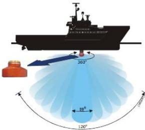
The HiPAP® 101 has a planar transducer array with a cylindrical body including 31 transducer elements. This model has good accuracy in the  $\pm 60^\circ$  coverage sector and is suited for operations where the major positioning targets are within this sector.
