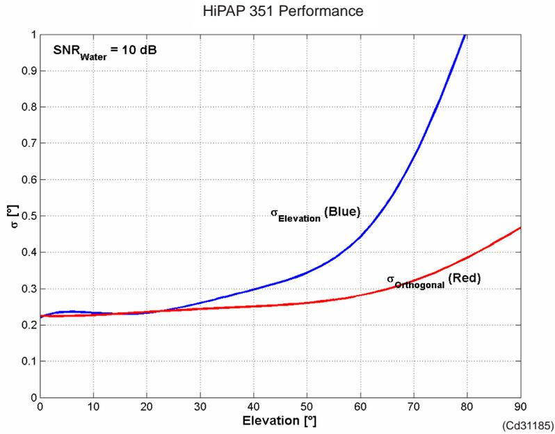
The figure above shows the accuracy as a function of elevation angle. The signal to noise ratio 10 dB is in the bandwidth.
