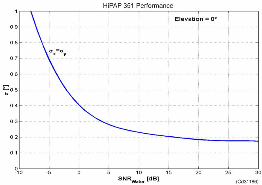
The figure above shows the accuracy as a function of signal to noise ratio. The elevation and the orthogonal angles are 0° (at vertical).
