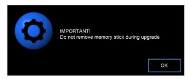
*Caution:* If the memory stick is removed before prompted by the system, the upgrade will fail and leave the Seapath system in an indeterminate state.
