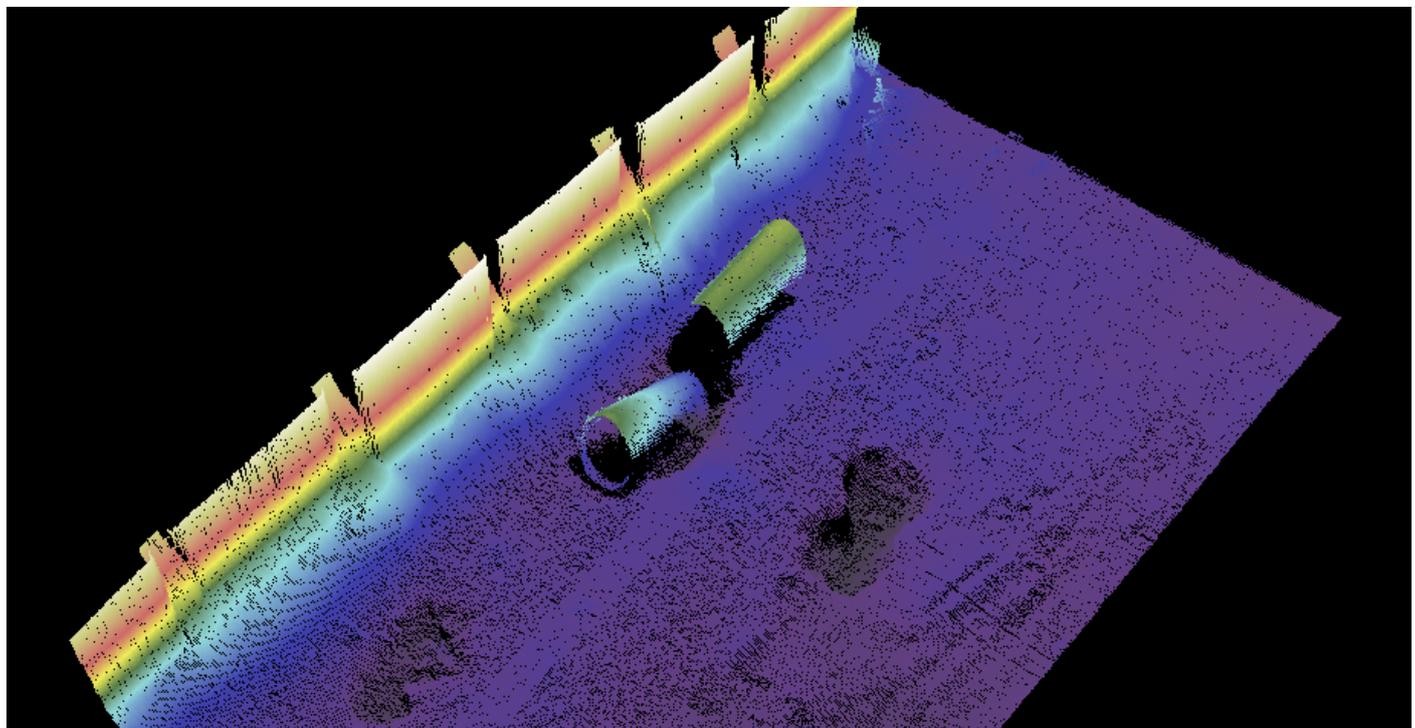
The **TOPAS PS 120 Parametric Sub-bottom Profiler (PSBP)** is the first portable PSBP in the TOPAS series. The system is designed for very high spatial resolution sub-bottom profiling in water depths from 2 meters to more than 400 meters
