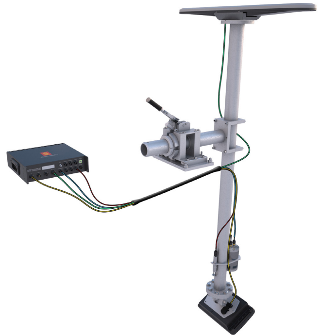
Pole connection diagram including the transducer, EM2040 processing unit and Seapath position, attitude, time and heading sensor. (Pole design for illustration purposes)
