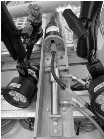
The transducer needs to be protected during launch and recovery of the ROV. It is also important to get a good line of sight to the LBL transponders while the ROV is navigating close to the seabed. This can be solved by using a hydraulic ram to raise and lower the transducer as needed.
