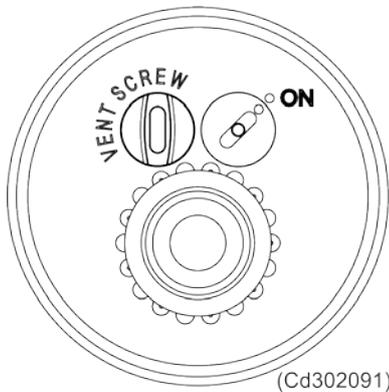
The ON/OFF switch has 4 positions. The subsea transceiver is only switched ON when the two marker dots are aligned. All other positions are OFF.
