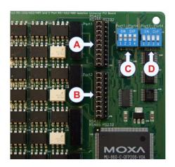
Table 1 Serial lines jumper and DIP switch settings
