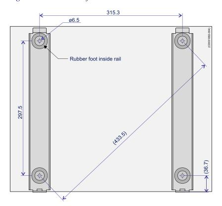
Figure 3 Installation of the Processor Unit
