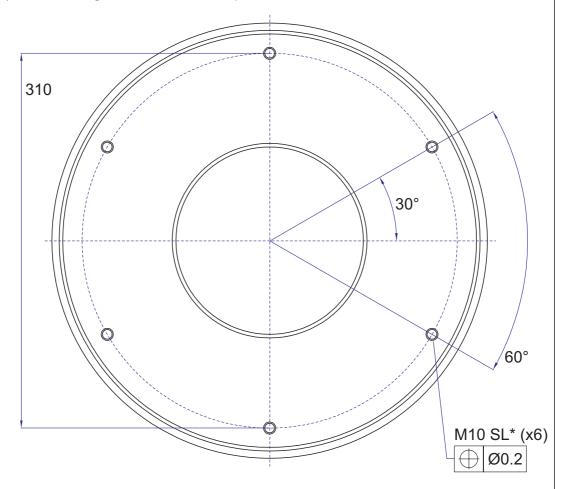
The self-lock threads (SL\*) must be made in accordance with Simrad procedure 842-202125. Self-lock taps can be supplied by Simrad.
