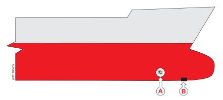
Recommended location of the transducer on a bulbous hull:
