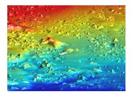
Figures: The Ormen Lange field survey. Data processed from EM 3000 on NUI Explorer.
