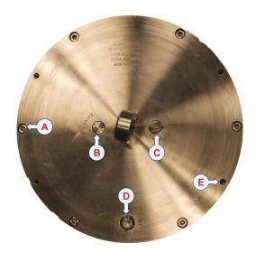
Insert longer M6 screws in the 6 holes, E to push open the lid.
