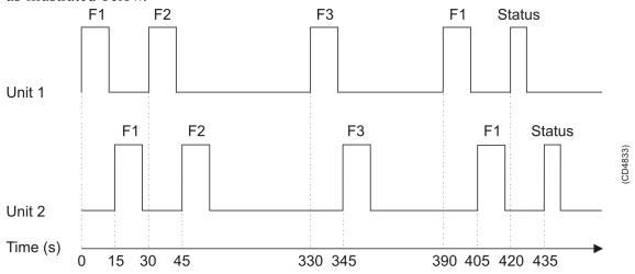
The sequence in the example with 4 single valve operations will be executed directly after triggering from the sensors from SCU 1. The SCU 2 will perform a defined delay before starting the ASHD valve sequence, trying to avoid that the SCU's are sending current to one solenoid at the same time.
