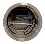
Insert the new battery.Inserting the battery at an angle makes it easier.
