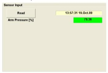
Tap **Read** to get new readings from the sensors. The time of the reading comes up and the colour of the field indicates if the values are within the set parameters.
