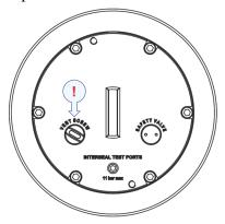
3 Use two longer M6 screws for extraction. Insert the screws into the extraction holes on the top of the unit and screw until the lid is open.
