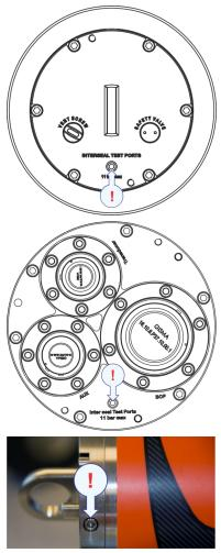
In addition this model has test ports on the connectors, to make sure these also are watertight. All must be tested at least every year.
