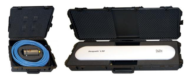
The Seapath 130 series is developed specifically for hydrographic surveying where high precision heading, position, roll, pitch, heave and timing are critical measurements. The product combines state-of-the-art dual frequency GNSS receivers, inertial technology and processing algorithms in a compact and portable package.
