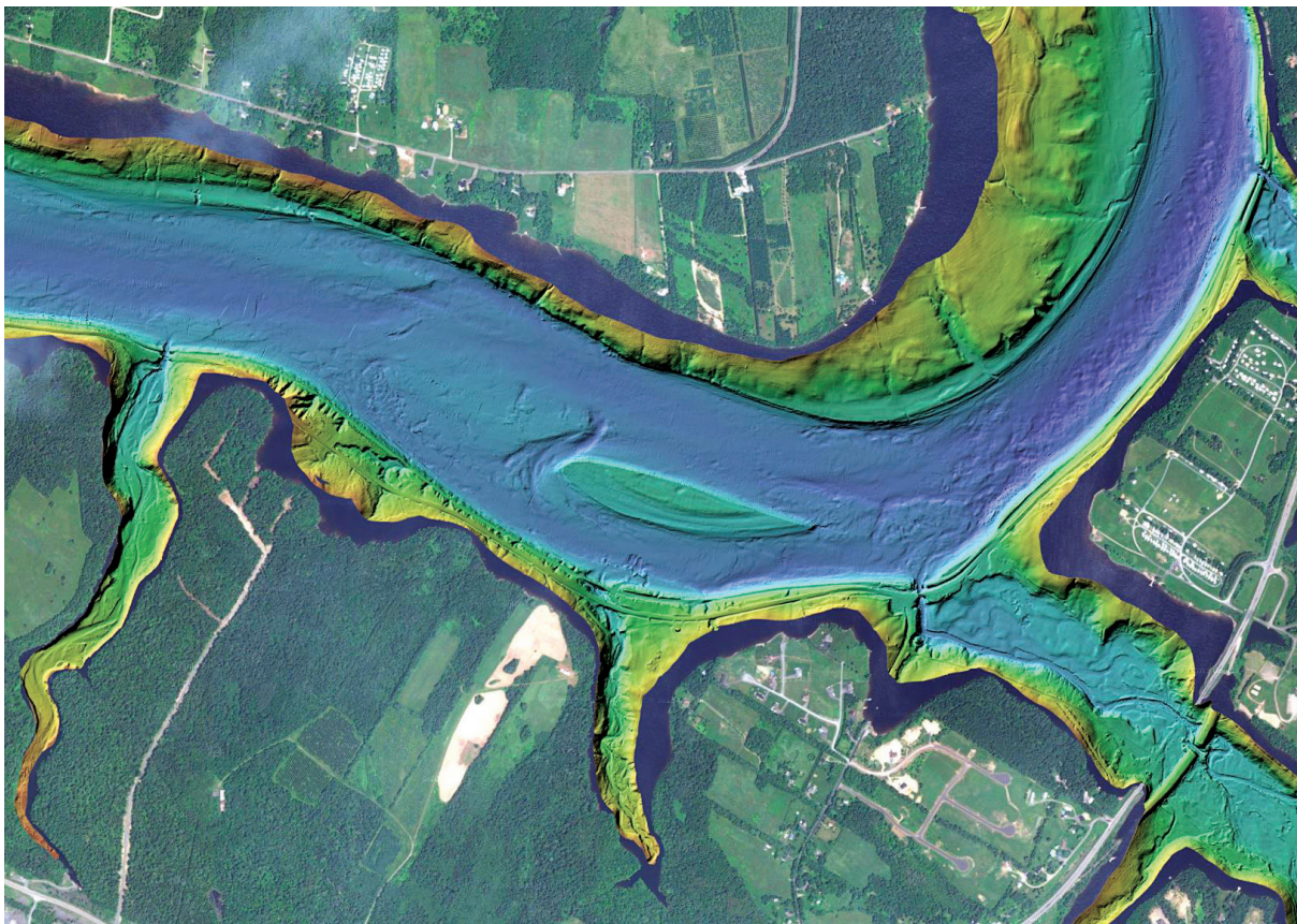
M3 Sonar - Bathymetric Capture, Maqtacquac Headpond Survey. Image courtesy of UNB-Ocean Mapping Group.
