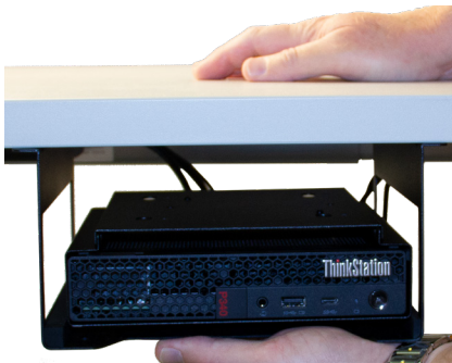
Installing VESA-box under the desk
