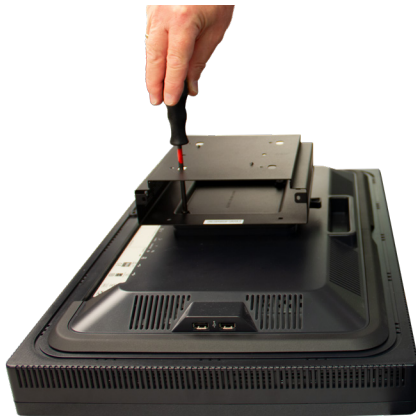
Installing VESA-box behind the display
