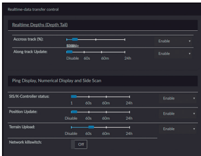
SIS Remote can be configured to transmit more or less data depending on the bandwidth available
