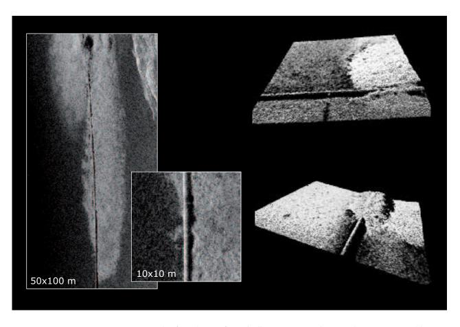
Example of SAS images from pipeline survey operation. 2 nmi x 500 m covered in one hour, with heavy overlap and one pass at each side of the pipeline
