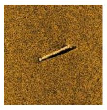
Standard FOCUS streaming SAS image (20 m  $\times$  20 m) of torpedo at 90 m range.
