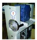
3 Move the hand crank to the hoist motor shaft.
