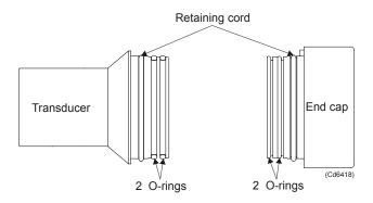
Figure 2 O-ring locations on transponder
