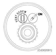
The ON/OFF switch has 4 positions. The subsea transceiver is only switched ON when the two marker dots are aligned.
