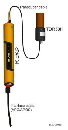
Figure 1 cPAP 34 with TDR30H
