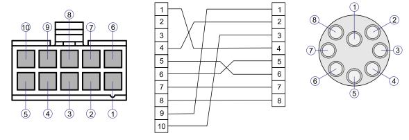
This is the Molex plug seen from the back where the crimp terminals are installed and a face view of the connector.
