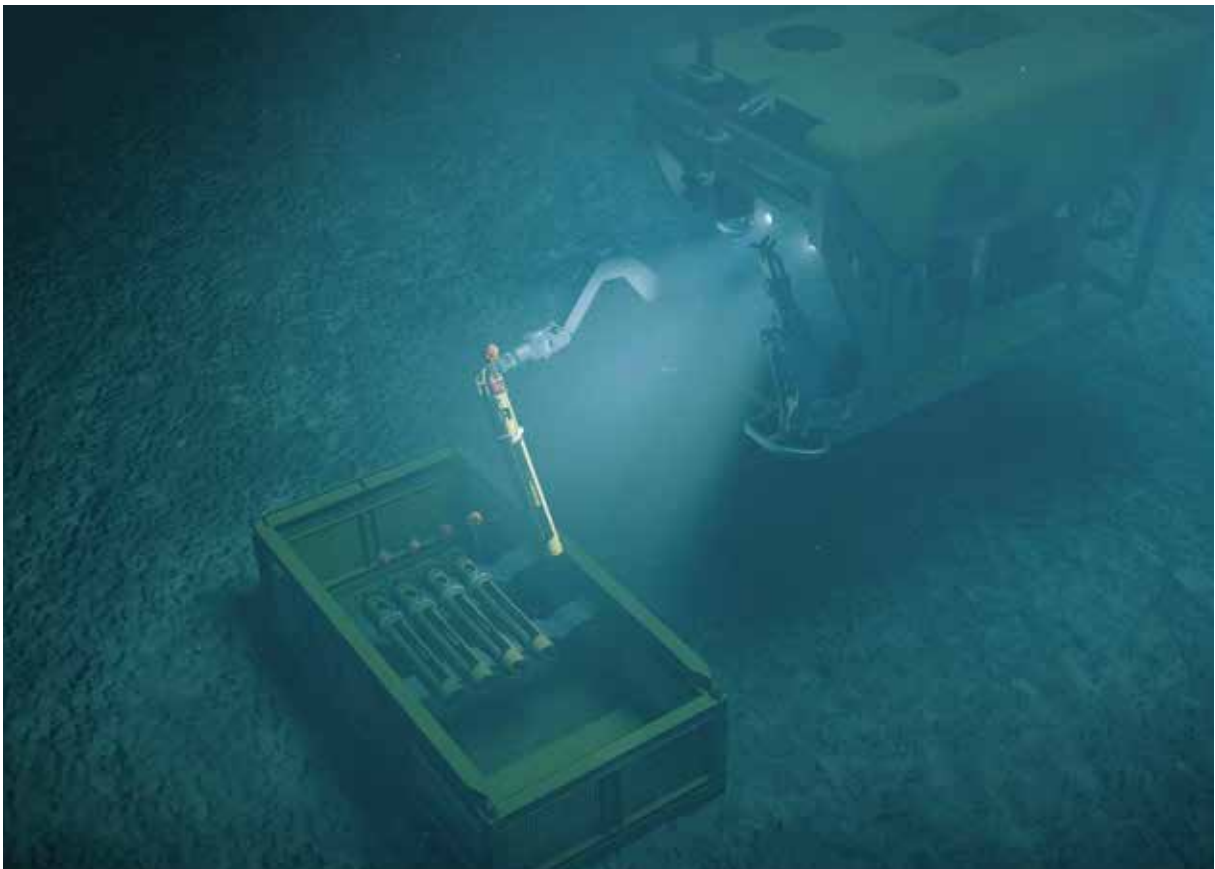
ROV deploying cNODE transponders with sensor module
