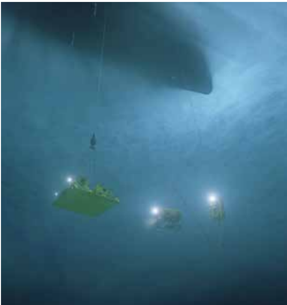
LBL structure placement via ROV cPAP transceiver
