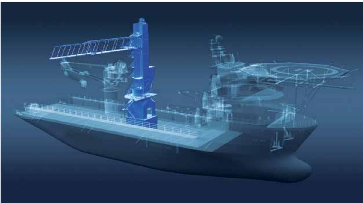
During the operation, the most significant ship systems in use are the gangway including access systems, the propulsion/thruster/steering systems and the energy production systems. Maneuvering and positioning control systems, the gangway control system and the integrated automation system including energy management control and coordinate operation of the ship equipment.
