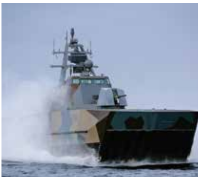
The Skjold class Corvette is one of the fastest warships in the world with a capability of speeds above 60 knots.
