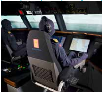
Royal Norwegian Navy is using a customized Kongsberg Digital simulator solution, which is a 1:1 simulator replica of the tactical bridge system on board the Skjold class Corvette.
