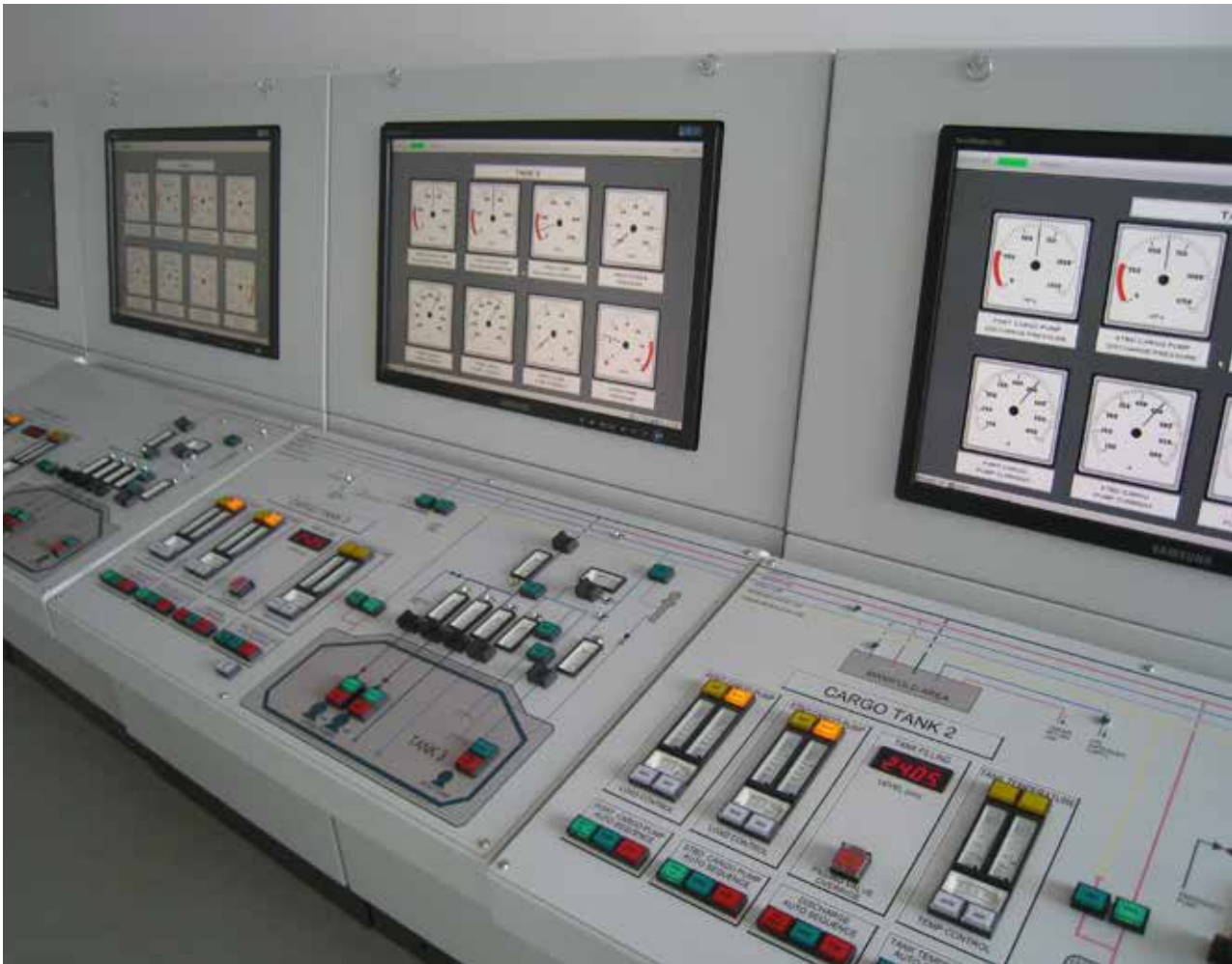
K-Sim Cargo, full mission version with operational panels and consoles for hands-on experience
